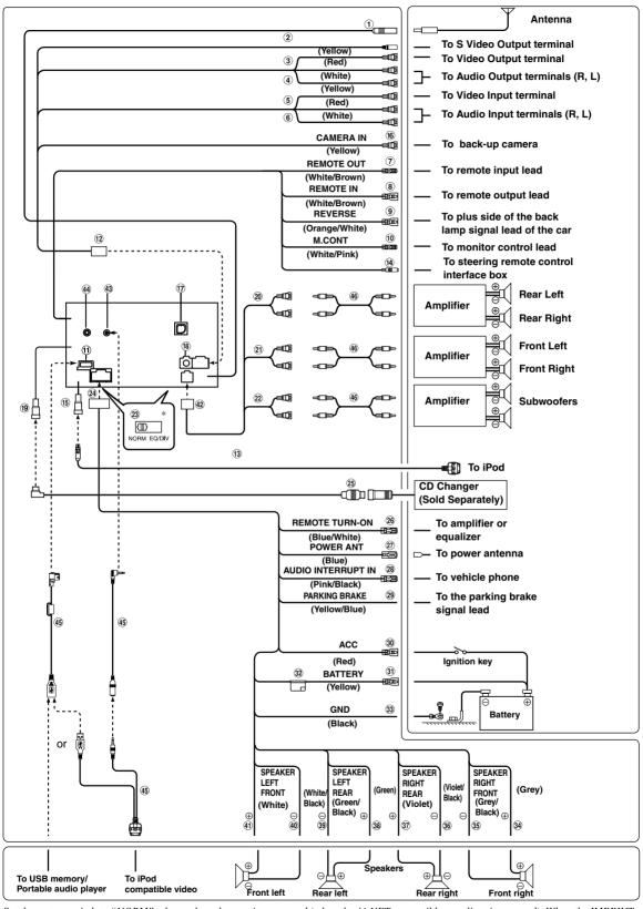
Set the system switch to "NORM" when only a changer is connected (when the Ai-NET compatible equalizer is not used). When the IMPRINT audio processor is connected, set to EQ/DIV position.
